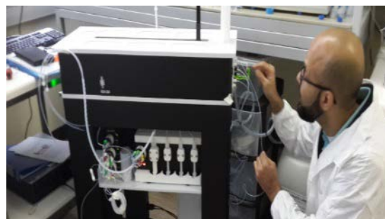
3A pico-Fast® system has been acquired for pre-concentration of sea-water samples for trace elemental analysis using ICP-MS. The system is now installed and validated for measurement of bioactive trace elements.
